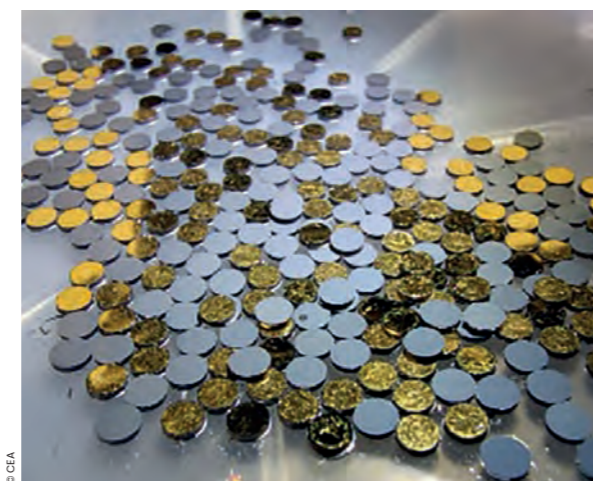
Figure 1: Boron-doped diamond electrodes produced at CEA-List using microwave plasma-assisted chemical vapor deposition.
